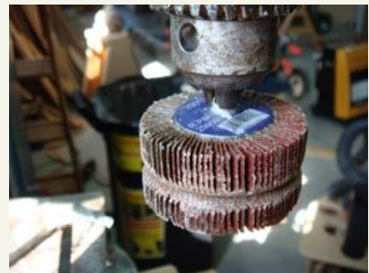
Figure 2: Sanding drum after first dipping in wax. The groove was cut prior to the second dipping.
